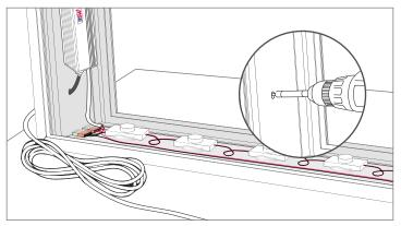
6 Drill holes on lightbox connect to the power supply.
