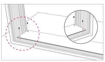
**2** Before installing the LEDs, screw the ACM panel to the bottom of the extrusion bar frame.
