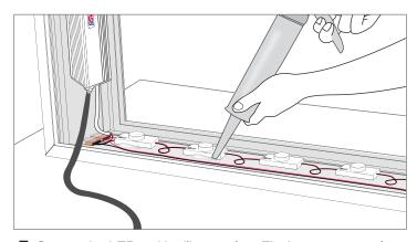
**5** Secure the LEDs with silicone glue. Fix the power supply to the inside of the lightbox with screws, and wire both ends of the LED modules to the power supply (refer to page 2)
